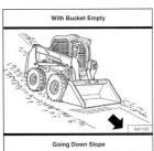
Always fasten your seat belt and follow other precautions that keep you inside the ROPS (protection cage). Failing to do so could allow ejection from this protective area result in death or injury including the tractor crushing you. NEVER allow riders anywhere on the machine!
